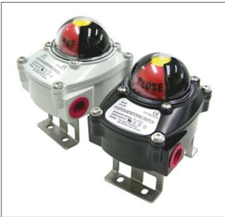
ITS series position monitoring switch boxes are primarily a rotary position indication device designed to integrate valve and NAMUR rotary pneumatic actuator with a variety of mounting options, internal switches or sensors and configurations.
